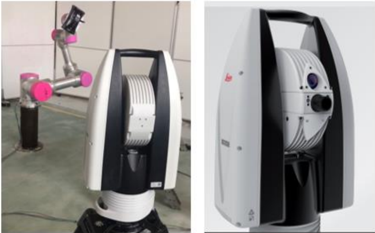
Figure 4.1 Experimental setup and the Leica laser tracker
